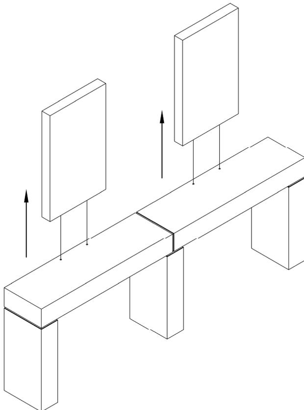
3. Carefully turn unit onto legs, adjust feet to ensure units are level. Attach Mirror Section (A) from underside of unit using M8 Bolts and Washers (E&F) provided. Repeat same process for any unit containing more than 1 Mirror Section.
